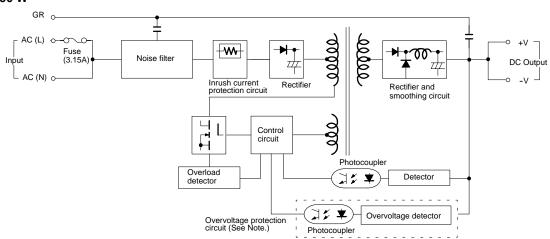
Note: Only the S8E1 with an output of 5 V incorporates an overvoltage protection circuit.
