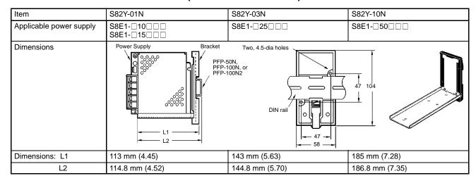
Note: The figures in row L1 are applied if a mounting bracket is attached to the power supply. The figures in row L2 are applied if either PFP-50N or PFP-100N DIN rail is used. Add 10.5 mm to each figure in the L1 row if PFP-100N2 DIN rail is used.
